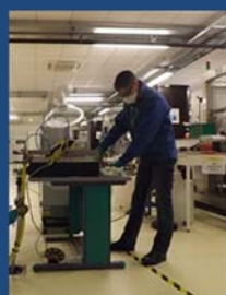
Condenser and water jet test for coating cleanability evaluation
