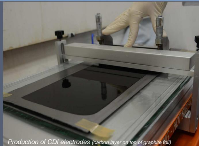
Production of CDI electrodes (carbon layer on top of graphite foil)
