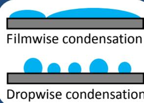
As water continuously condenses, drops slide down and grow by coalescing with all other drops in their path. These drops leave a wet trail on metal surfaces, but an initially dry trail on hydrophobic surfaces until new condensation starts.
