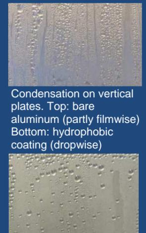
Condensation on vertical plates. Top: bare aluminum (partly filmwise) Bottom: hydrophobic coating (dropwise)
